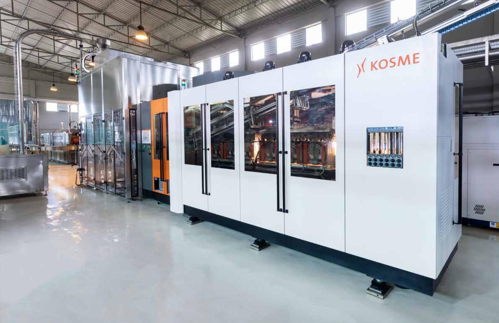
In the SynchroBloc a Kosme KSB 8R blow-moulder is block-synchronised with a Kosme Volufill filler.
